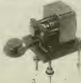
Fig. 7. Improved Receiving Variometer Having Three Windings, Connected to a Special Switch Permitting of Series and Parallel Combinations of the Coils. Coils are Wound Self-Supporting.
