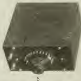
Fig. 6. A Variable Step Inductor for Use in Audion Regenerative Circuits. Coupling is Possible by Placing One Coil Box On Another. Has No-End-loss Switch.
