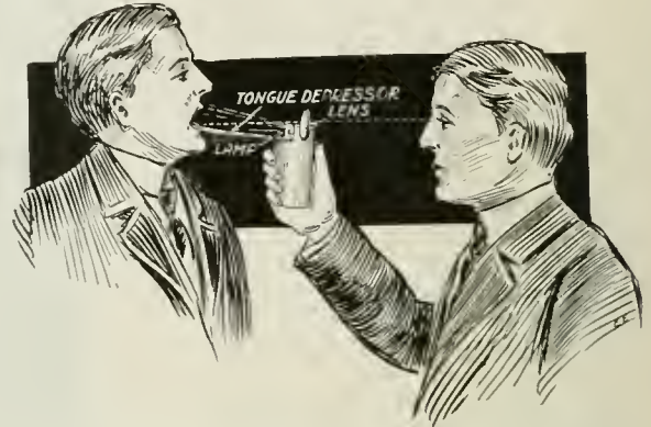
A Recent Invention Comprises a Diagnostic Lamp, Lens, and Tongue Depressor All in One Instrument.
